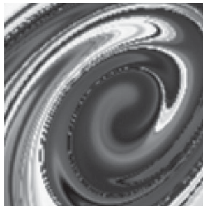
FIGURE 2. The x - y plane cut at z = \pi from the three-dimensional Lagrangian scalar field at t = 2.5T_e with the initial condition \phi_0 = \cos x in the forced stationary homogeneous and isotropic turbulence, and zoomed parts of plane cuts at a small region 2.5 \leq x \leq 2.9 and 3.6 \leq y \leq 4 with increasing resolutions.
