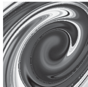
FIGURE 2. The x - y plane cut at z = \pi from the three-dimensional Lagrangian scalar field at t = 2.5T_e with the initial condition \phi_0 = \cos x in the forced stationary homogeneous and isotropic turbulence, and zoomed parts of plane cuts at a small region 2.5 \leq x \leq 2.9 and 3.6 \leq y \leq 4 with increasing resolutions.
